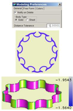
The (obvious) advantage to modeling gerotor profiles with "expressions" is parameterized section geometry.
